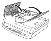
Raise the roller unit's lock lever. (Gently bend the lock lever inward, then raise it.)
